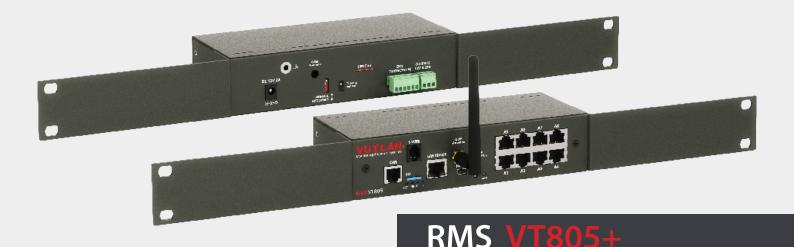
The unit is used for environmental control in different facilities. Can connect up to 30 sensors, 4 dry contacts, two 12V alarm beacons, GSM modem, USB camera, four IP cameras, SD card for logs, 1-Wire board with 1-Wire sensors. Has a built-in web interface & supports protocols like HTTP, HTTPS, SNMP v1, 2c, 3, SMTP, Radius, Syslog and other.
